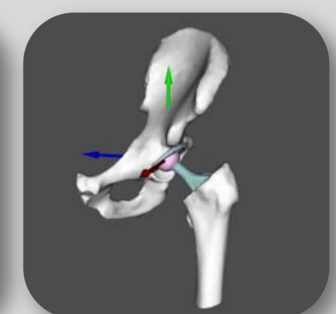
Prosthetic hips developed using CAD software with variations of cup positioning
